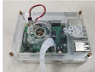
**Figure 13.** Raspberry Pi-based edge node
